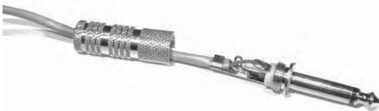
Figure 7.4 Cable soldered to plug.
