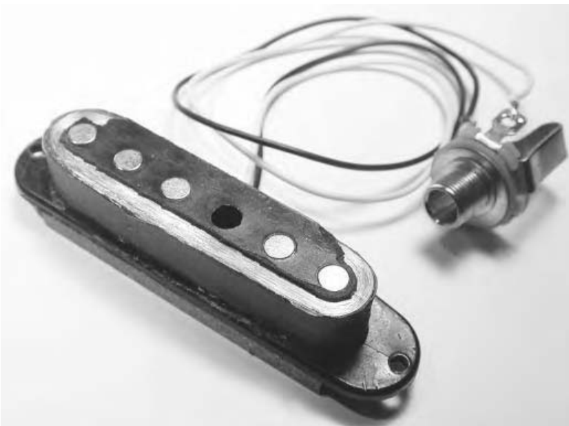
Figure 3.2 A guitar pickup with case broken away to reveal internal coil.
