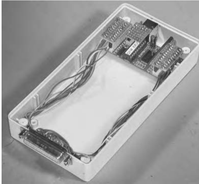
Figure 29.2 Sensor-to-USB interface built with CH Products interface board (open).
