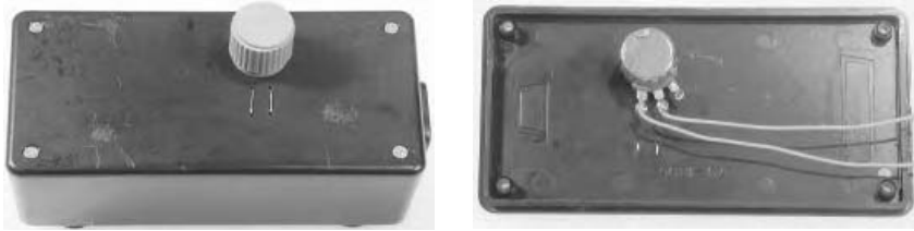
Figure 15.7 A potentiometer with electrodes in parallel.
