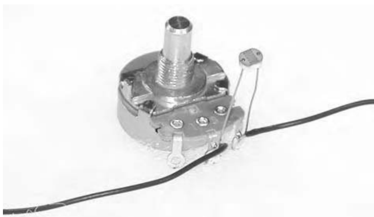
Figure 15.5 A potentiometer and photoresistor in parallel.
