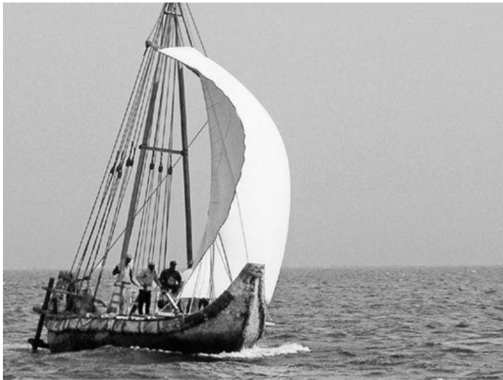
The Magan Boat, a modern interpretation of an Omani ocean carrier of the late third millennium BCE built in 2005. The A-frame mast distributes the downward pressure across the reed bundles that form the hull. The reeds are made waterproof by the application of a bitumen amalgam, the recipe for which was derived from fragments of ancient sheathing found near Ras al-Jinz, the easternmost point of Oman on the Arabian Sea. Courtesy Tom Vosmer.
