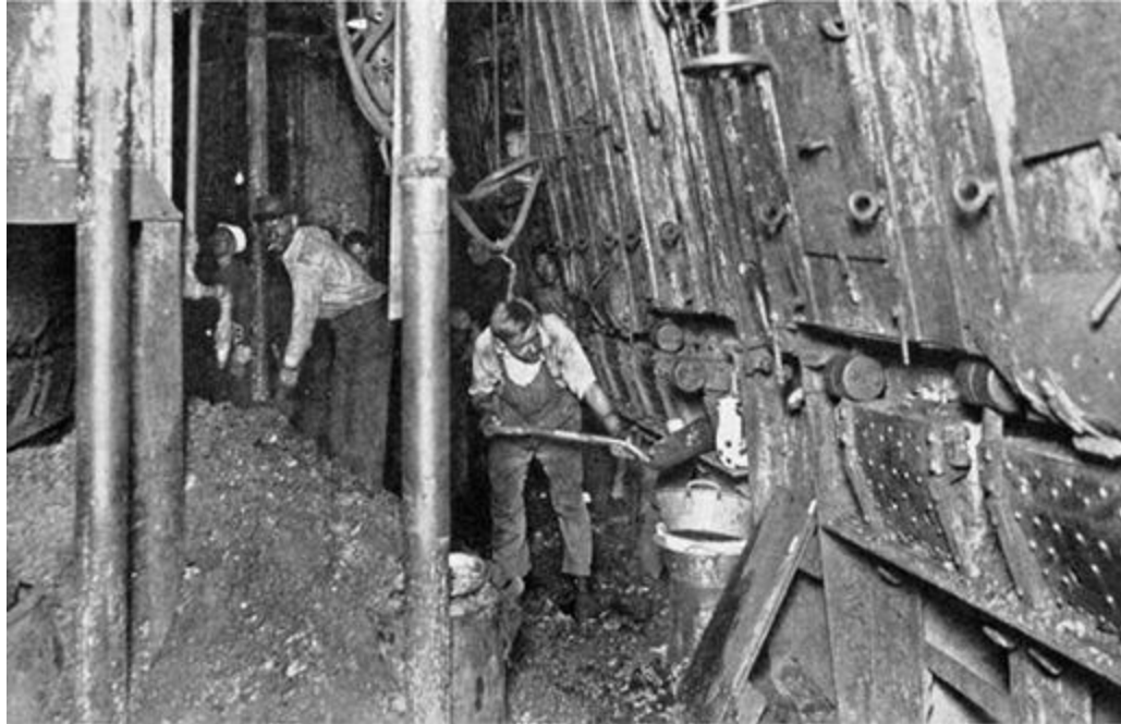
Built for transpacific service between Seattle and Shanghai, the Great Northern Steamship Company's passenger freighter Minnesota was driven by a pair of triple-expansion steam engines whose insatiable demand for coal made for unrelenting toil by the ship's stokers. This photograph was taken while the ship was under charter to the U.S. Navy as the troopship USS Troy (there was already a battleship USS Minnesota) during World War I. But the conditions in the inferno belowdecks in steamships remained the same regardless of the ship's mission. Courtesy of the U.S. Naval History and Heritage Command, Washington, D.C.
