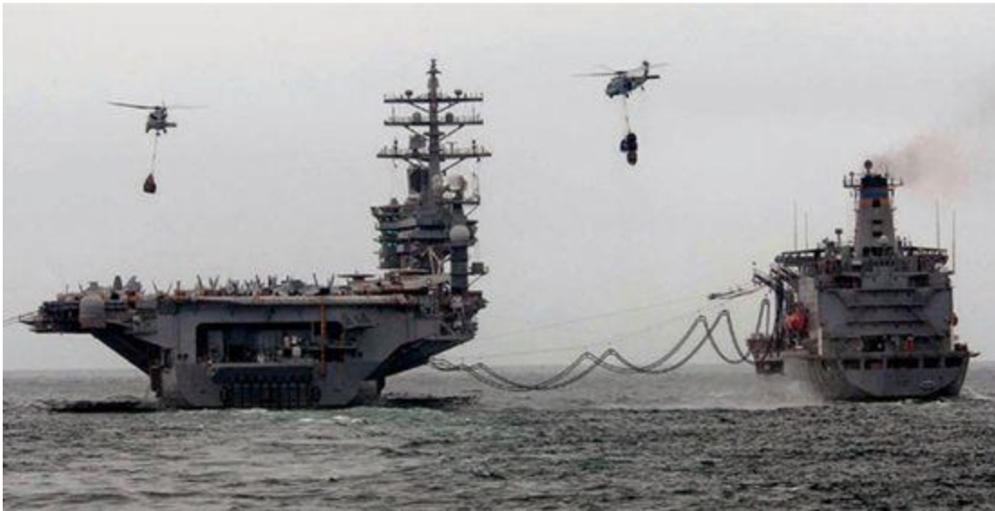
26. The Nimitz -class aircraft carrier USS Dwight D. Eisenhower being replenished by the fleet oiler USNS Big Horn . The Eisenhower is nuclear-powered and the hoses leading from the Big Horn supply jet fuel for the carrier's air wing, while helicopters transship dry goods, including mail for the crew. The U.S. Navy has long been in the vanguard of underway replenishment, which is essential to long-distance overseas operations such as those shown here in the Arabian Sea. Photograph by Darien G. Kennedy; courtesy of the U.S. Navy.
