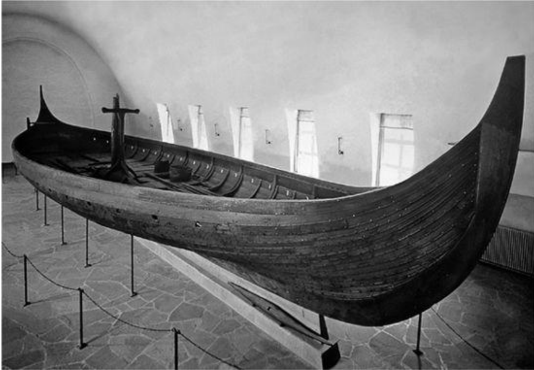
The Gokstad ship of 895 is a large clinker-built karvi intended for ocean sailing. Built primarily of oak, the hull measures twenty-three meters by five meters and could carry about sixty-five people. The ship was found in a burial mound near Sandefjord, Norway, with three smaller boats, a bed, cooking implements, and twelve horses, six dogs, and other animals. Courtesy of the Vikingskipshuset, Oslo.
